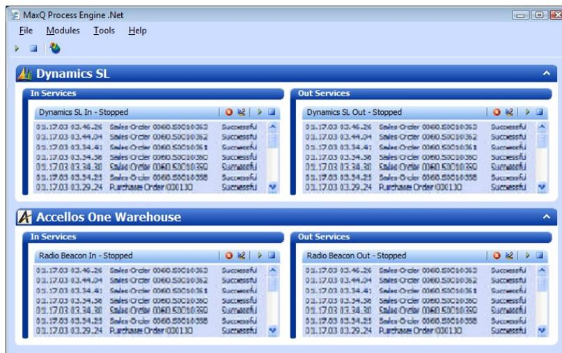
*The Warehouse Interface Control Center is the heart of Accellos One Warehouse Link for Dynamics SL. This .NET service handles all the interfacing of information between Dynamics SL and the Accellos One Warehouse WMS. It provides a very flexible and scalable solution.*
